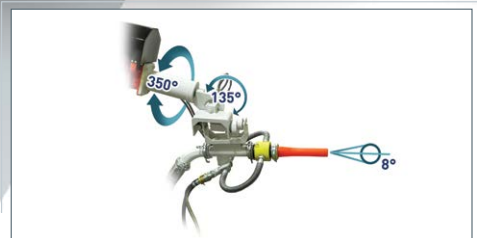
350° rotation +/-135° tilt and 8° oscillation spraying head
