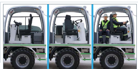
ROPS and FOPS level 2 certified closed operator cabin with 180° pivoting operator's seat
