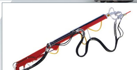
Robust manipulator with 10 m vertical and 8 m horizontal spraying reach
