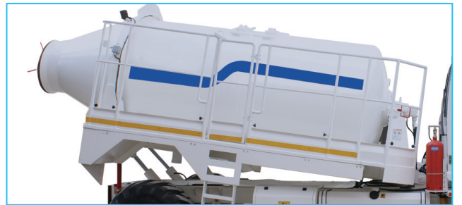
Hydraulic drum tilting up to 8°
