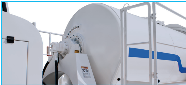
Horizontal drum with 5 m 3 concrete yield
