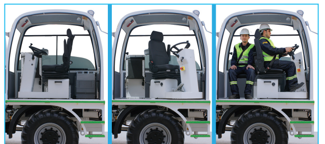
ROPS and FOPS level 2 certified closed operator cabin with 180° pivoting operator's seat
