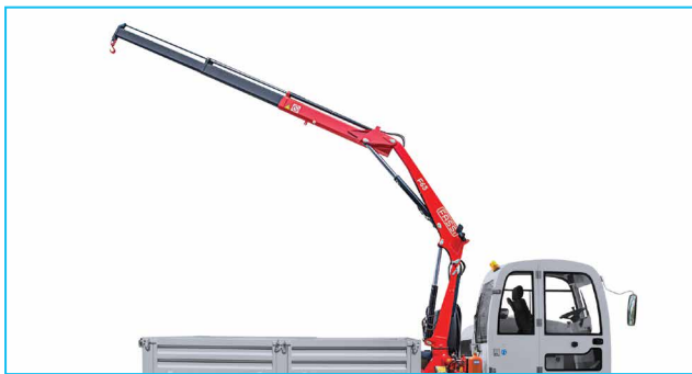
820 kg lifting capacity at 7.1 m
