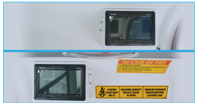
Rear view camera and LCD screen in operator cabin
