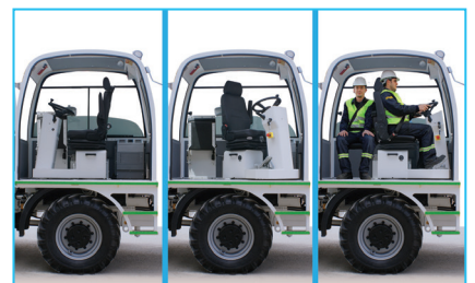
ROPS and FOPS level 2 certified closed operator cabin with 180° pivoting operator's seat
