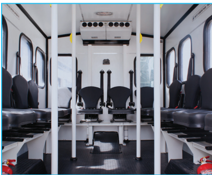
ROPS and FOPS level 2 certified closed personnel cabin
