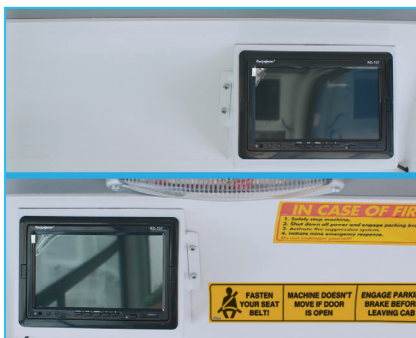
Rear view camera and LCD screen in operator cabin
