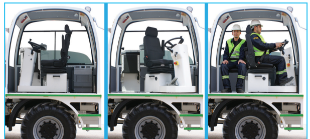
Closed cabin with 180° pivoting operator seat and ROPS & FOPS Level 2 certification
