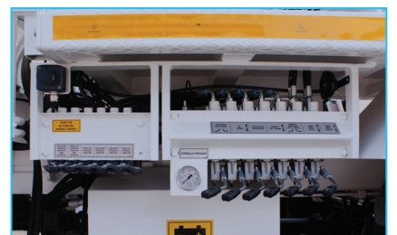
Boom, basket and stabilizers manual controls
