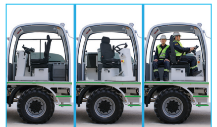
ROPS and FOPS level 2 certified closed operator cabin with 180° pivoting operator's seat
