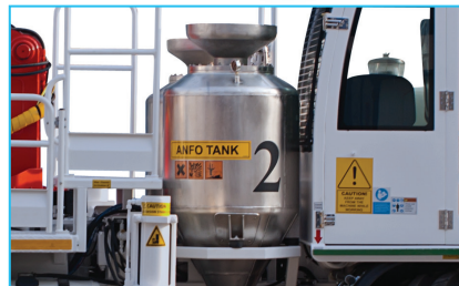
2 x 350 L capacity ANFO tank
