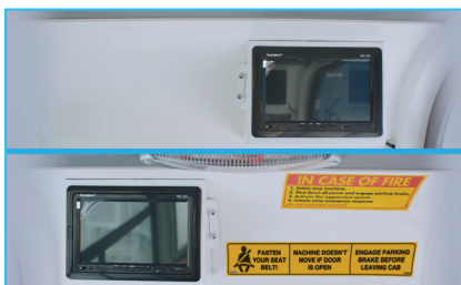
Rear view camera and LCD screen in operator cabin
