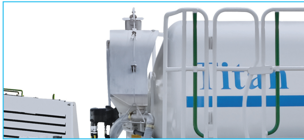
5.6 m 3 concrete yield 220 l stainless steel admixture tank (optional)
