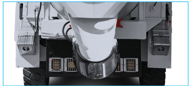
Hydraulically controlled shutter and chute
