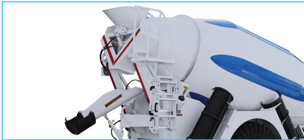
6 m 3 concrete yield
