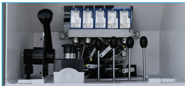
Platform and legs controllable from 2 panels
