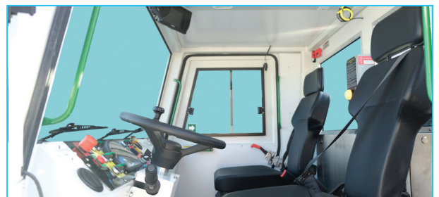
ROPS & FOPS level 2 certified closed 2-person cabin
