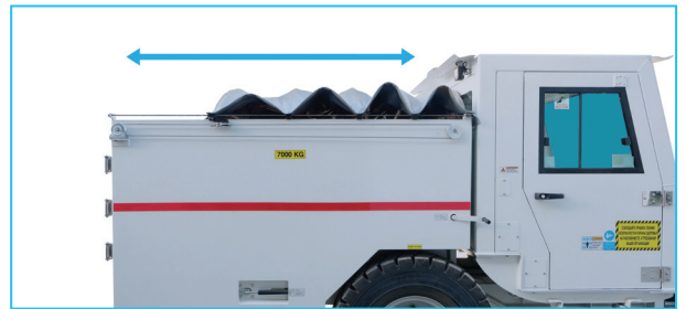
Manual opening / closing awning mechanism on the case
