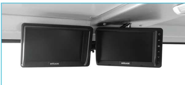
Rear view camera and LCD screen in operator cabin
