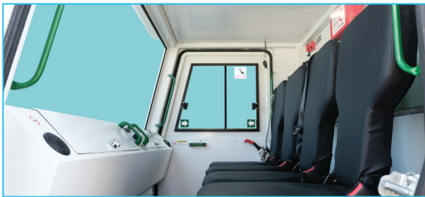
ROPS & FOPS level 2 certified closed 4-person personnel cabin
