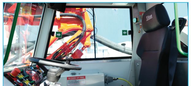
ROPS & FOPS level 2 certified closed 1-person cabin
