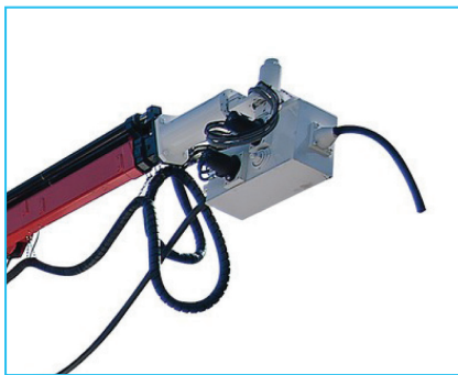
2 pcs remote controlled, hydraulically driven ANFO charging hose feeder
