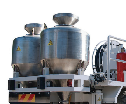
2 x 500 l stainless steel ANFO tanks
